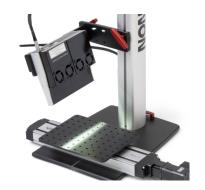
COBRA Hyperspectral LED: Very bright, stable, and long lifespan. VNIR cameras only, LED spectral range is 405-970 nm.
