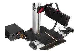
Halogen Fiber Line Light: Recommended for heat-sensitive samples and required for the Reflectance/Transmission System.
