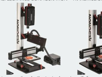
This system allows for illumination from above (Reflectance) or from below (Transmission). A clear sample plate is mounted to the linear stage and the line light easily transfers for the two configurations.
