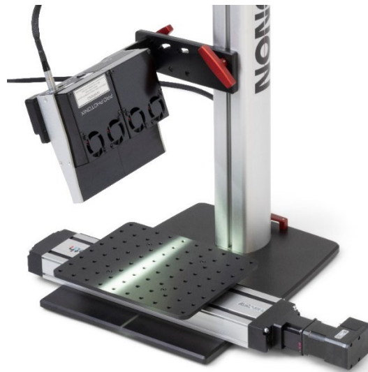
Figure 3. Benchtop Reflectance system with the Hyperspectral LED Light.
