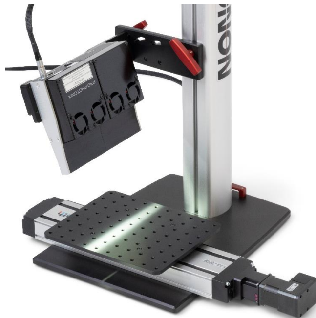
Figure 3. Benchtop Reflectance system with COBRA Hyperspectral LED light.
