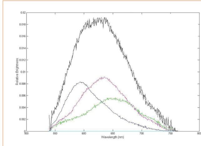
FLUORESCENCE SPECTRUM OF PROTEINS LABELLED WITH A MIXTURE OF THREE DYES THAT HAVE STRONGLY OVERLAPPING EMISSION SPECTRA (DATA CURVE, BLACK SOLID LINE) MEASURED WITH THE HYPERSPECTRAL IMAGER. THE DECONVOLUTED COMPONENT SPECTRA ARE SHOWN BELOW (COLORS) AND THE SUMMATION OF THE COMPONENT SPECTRA IS THE DASHED LINE OVERLAYING THE EXPERIMENTAL SPECTRUM.
